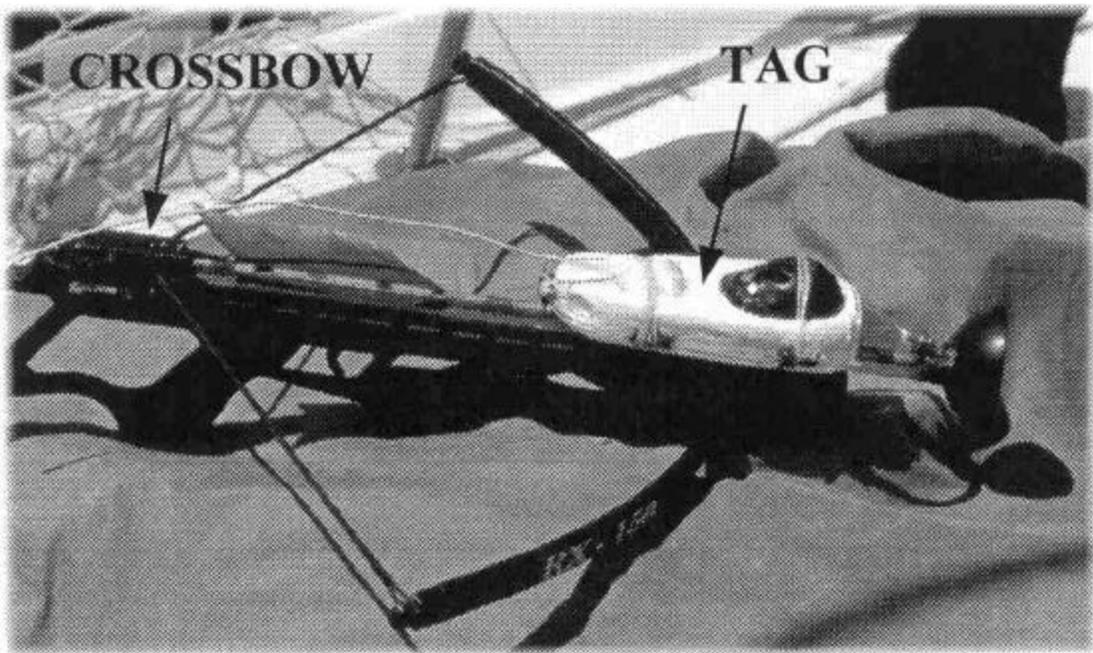
Figure A1.1. Suction-cup attached time-depth recorder/VHF radio tag ready to be deployed from the crossbow.
